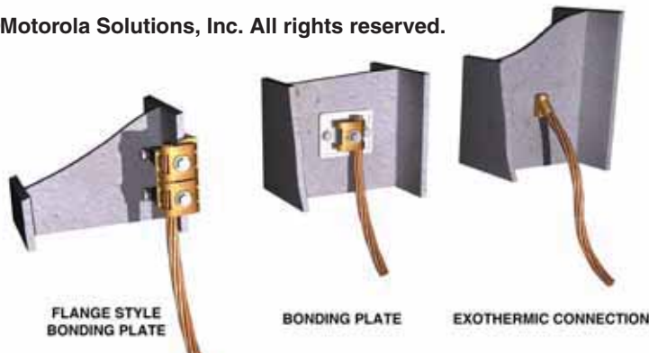
Figure 4-97 Acceptable Structural Building Steel Bonding Connections
