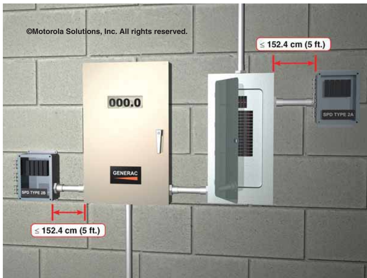
Figure 7-1 Minimum AC Surge Protection Installation Complement for a Typical Communications Site
