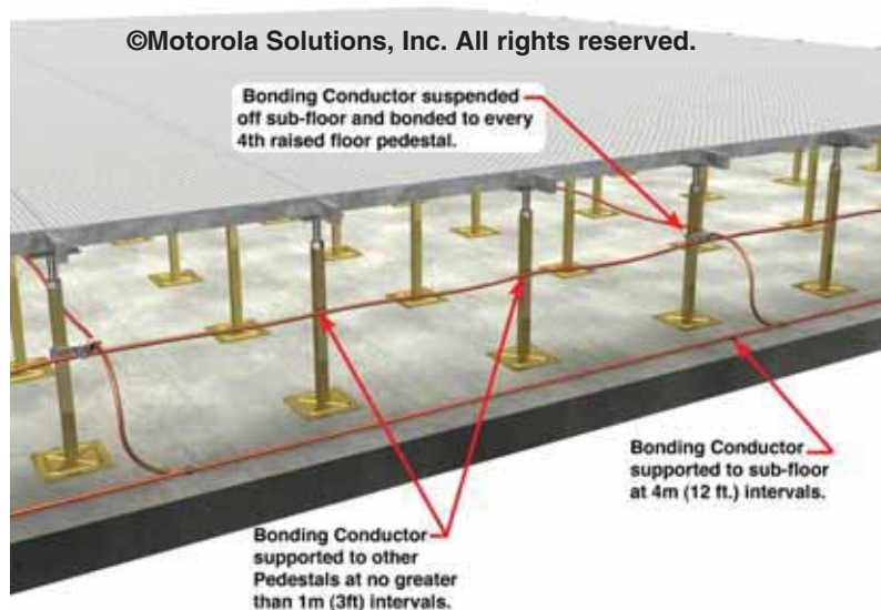
Figure 5-42 Securing Bonding Conductors Under Raised Flooring System
