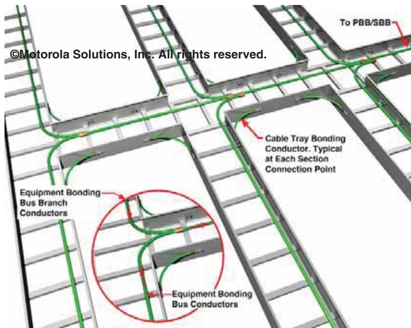
Figure 5-126 Example of Equipment Bonding Bus Conductors
