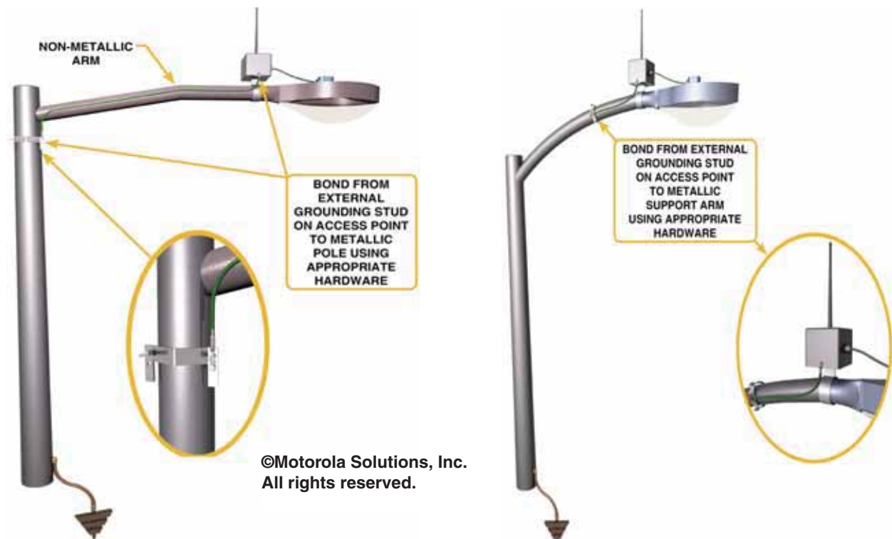
Figure 4-108 Grounding Access Point Mounted on Metal Pole
