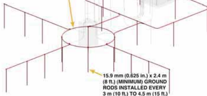
Figure 4-25 Example of Building and Tower Ground Ring With Radials
