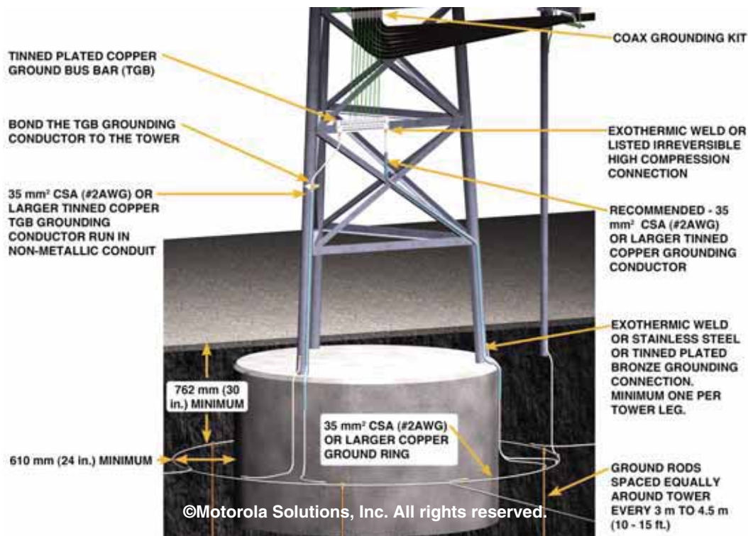
Figure 4-47 Bottom Tower Ground Bus Bar Configuration: Example 5
