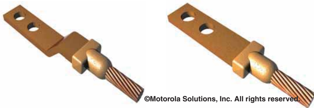
Figure 4-52 Lugs Exothermically Welded to Conductor
