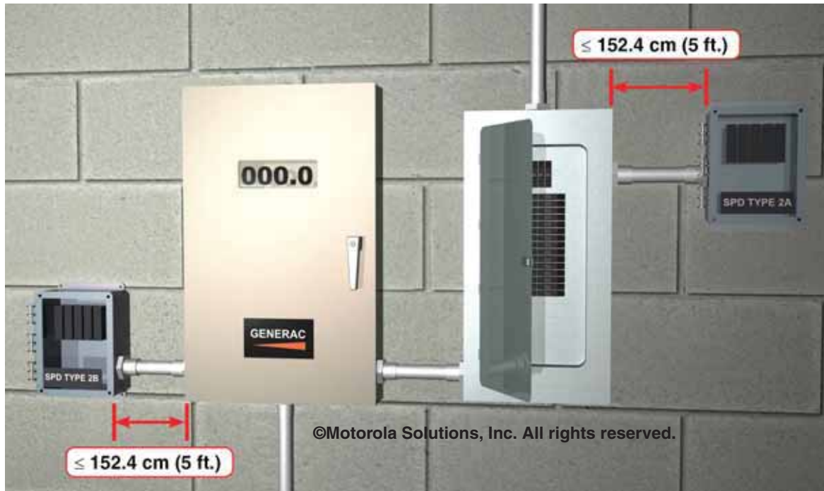
Figure 7-12 Example of SPD Conductor Length
