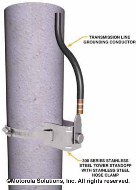
Figure 4-79 Grounding Transmission Line Top and Middle (Tubular Tower)
