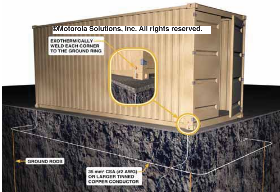
Figure 4-110 Grounding of Metal Shipping Containers
