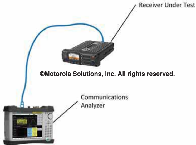
Figure G-36 Configuration for Measurement of Basic Receiver Sensitivity
