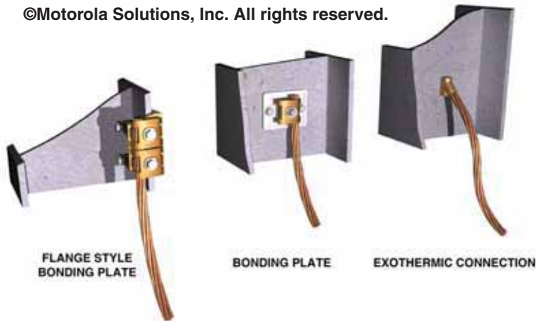
Figure 5-69 Examples of Acceptable Structural Building Steel Bonding Connections
