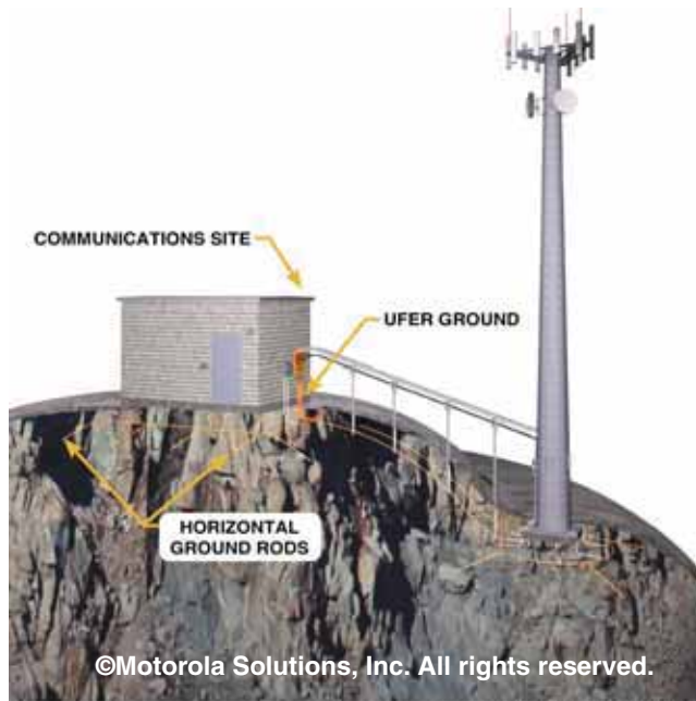
Figure 4-118 Installation of Horizontal Ground Rods in Shallow Topsoil Conditions
