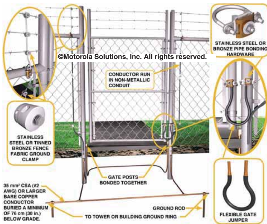
Figure 4-87 Example of Gate Bonding
