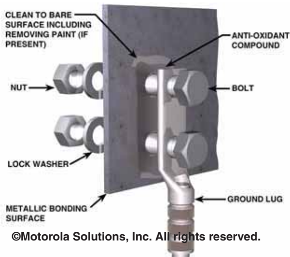
Figure 5-65 Proper Location of Washer When Connecting Ground Lug
