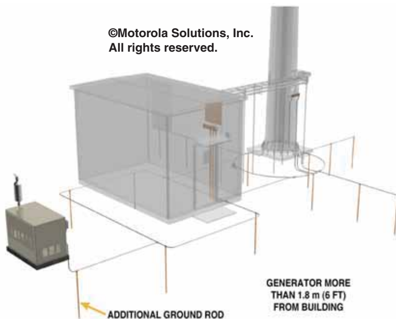
Figure 4-75 Generator Grounding: More than 1.8 m (6 ft) from Building
