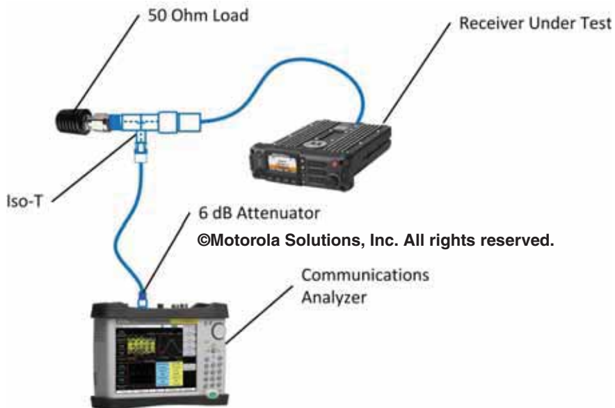
Figure G-37 Configuration for Measurement of Effective Receiver Sensitivity with 50 Ohm Load
