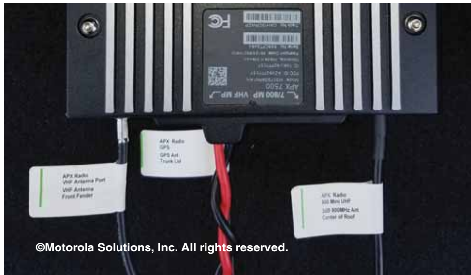
Figure G-8 Example of Coax Cable Labeling
