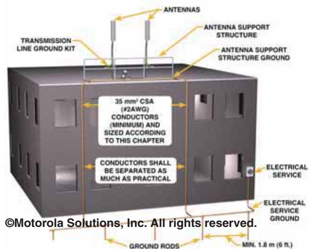
Figure 4-96 Roof Mounted Antenna Mast Grounding with Supplemental Grounding Electrode System
