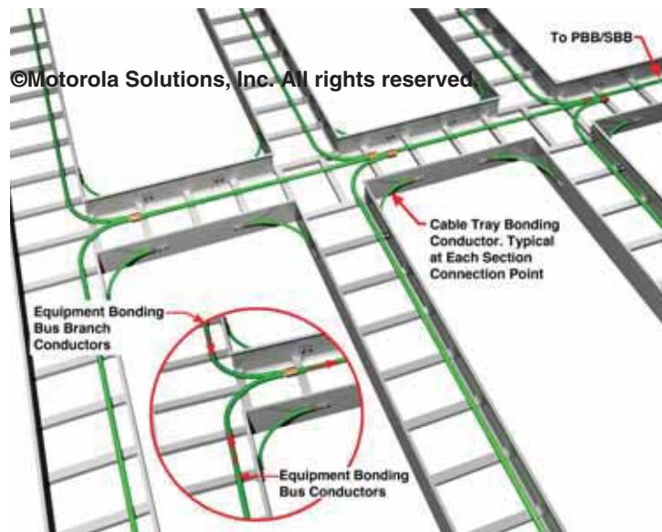
Figure 5-98 Example of Bonding Jumpers Installed on Cable Tray System (Top View)
