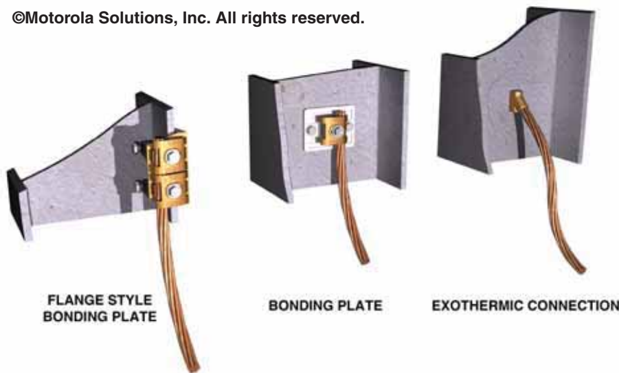
Figure 5-132 Examples of Acceptable Structural Building Steel Bonding Connections
