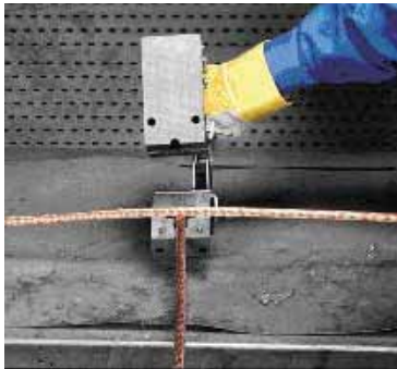
STEP 1: Clean and dry conductors and mold. insert conductors into mold.
