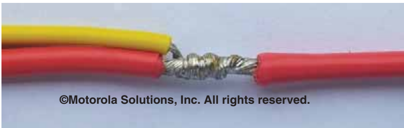
Figure G-24 Example of Completed Solder Connection
