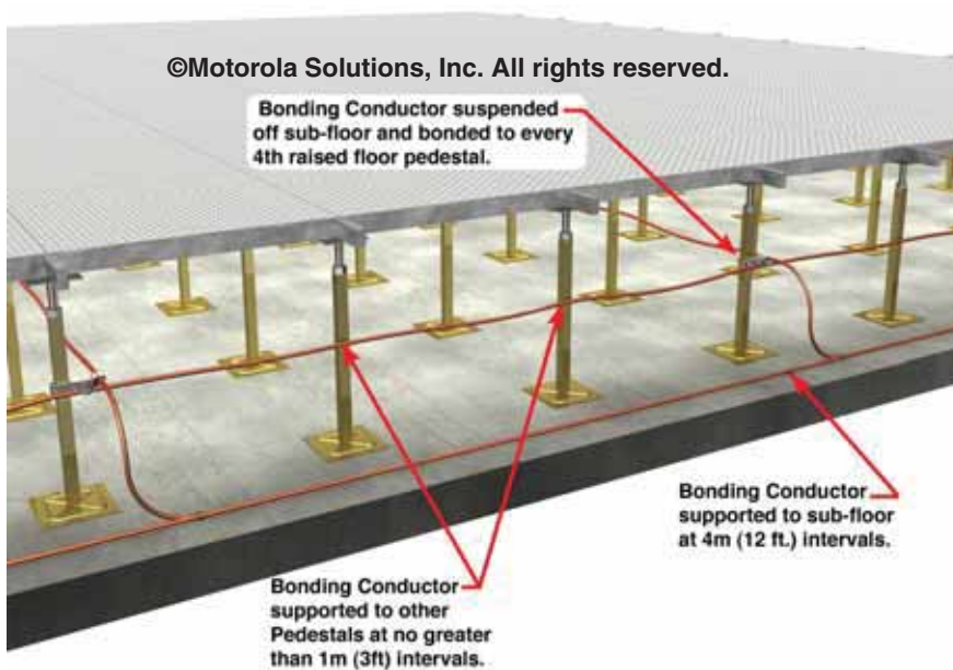
Figure 5-63 Example of Securing Grid Bonding Conductors Under Raised Flooring System
