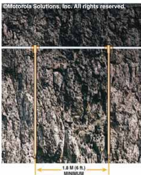
Figure 4-12 Parallel Ground Rod Installation
