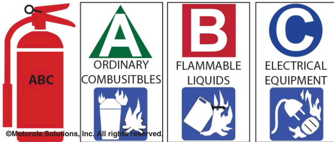
Figure 3-11 Fire Classification Labeling Examples
